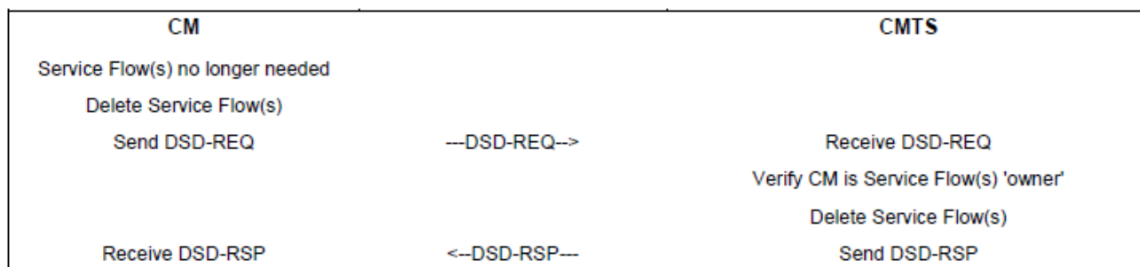
Figure 232 - Dynamic Service Deletion Initiated from CM
